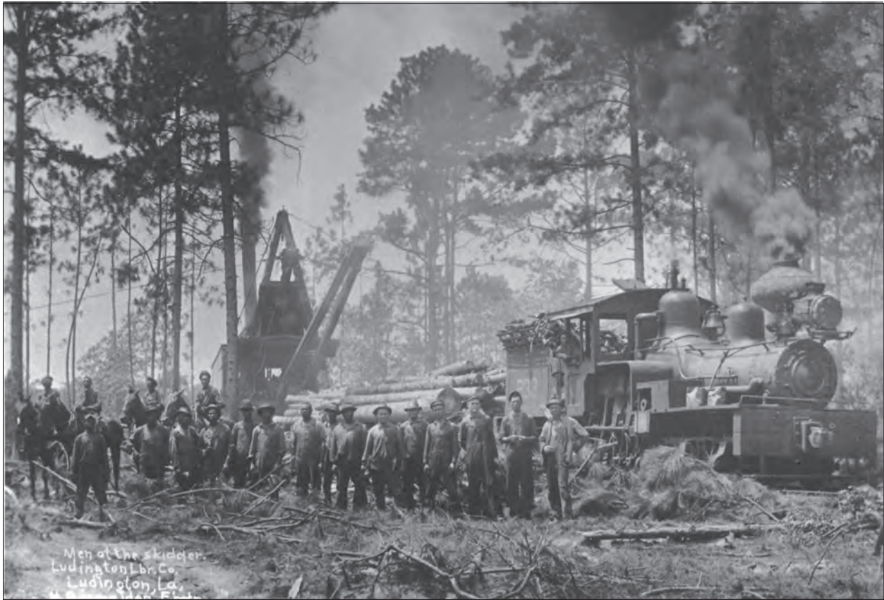
Figure 31 — Skidder, logging crews, and a Shay steam engine, Luddington Lumber Company (courtesy Museum of West Louisiana).
