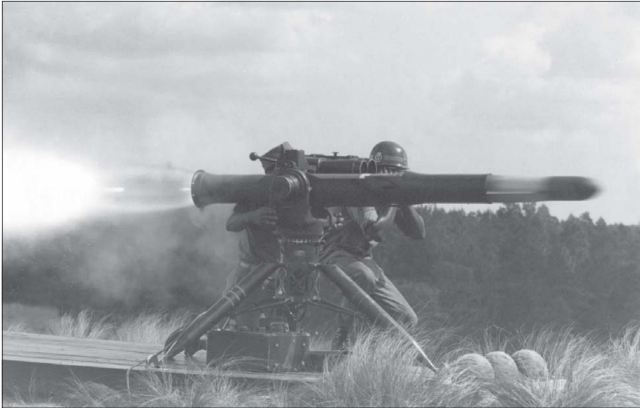
On September 11, 1975, during the Cold War, a soldier practices firing TOW (tube launched, optically tracked, wire guided) missiles in preparation for possible battle with the Soviet Union.
