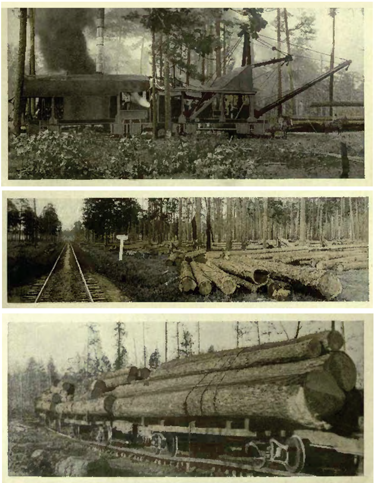
Figure 1-2.14. Top, a four-line skidder and loader handling logs at the rate of seventy million feet a year; Middle, longleaf pine logs assembled for loading; Bottom, logs on the way to the sawmill. Source: The Long-Bell Lumber Company (1920).
