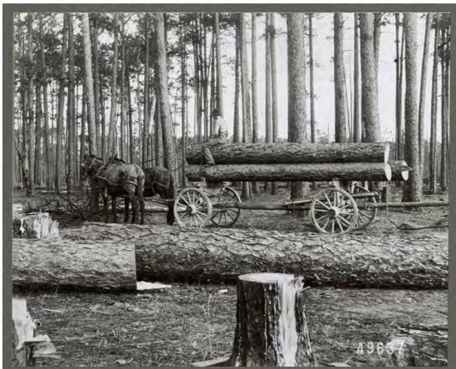
Figure 1-2.6. Carson, Calcasieu (now Beauregard) Parish. Taken by J. C. Peters, 1904. Original caption: "A skid wagon loaded with longleaf pine logs. A method of skidding logs, used either for short logs or long hauls." With the advent of steam logging, "[o]nce a man became part of the steam logging, he was considered superior to the poor logger with mule teams." Note: the northern portion of Calcasieu Parish, where the Carson mill was located, was incorporated into Beauregard Parish in 1913. Sources: Wise 1971:12; NARA 2014.
