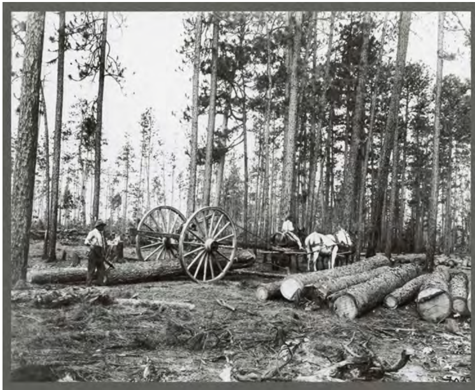
Figure 1-2.5. Pickering Lumber Company, Vernon Parish. Taken by E. J. Davison, 1903. Original caption: "Skidding Longleaf Pine logs out of the woods using Big Wheels." Source: NARA 2014.
